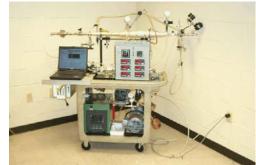
SwRI SPSS, Facilitate Solid Particle Measurement (Used Upstream of EEPS)
